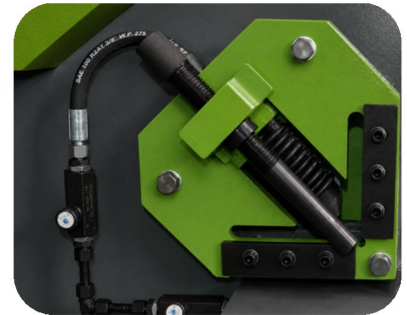
*Hydraulic hold-down for angle shear
