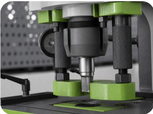
Standard dual-opening die block for up to 2" (50mm) round punch and die.
